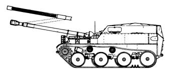
Figure 6-19. Self-propelled assault guns. Two types of light SP assault guns are employed by Soviet airborne troops. The ASU-57 (above), with a 57-mm anti-tank gun, has only light armored protection and an uncovered crew's compartment. Note the four large roadwheels. The newer 85-mm ASU-85 (below) is fully armored.
